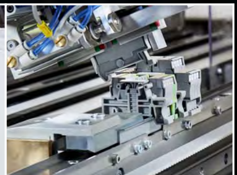
Automatic terminal block assembly
