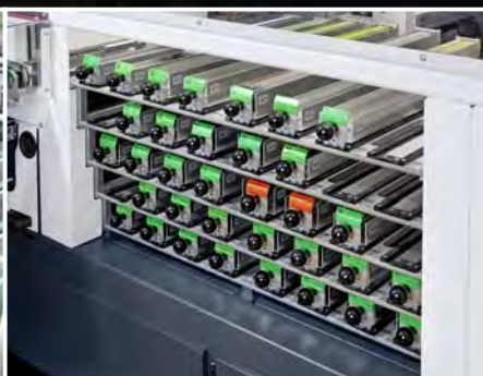
Magazine and magazine support for terminal blocks
