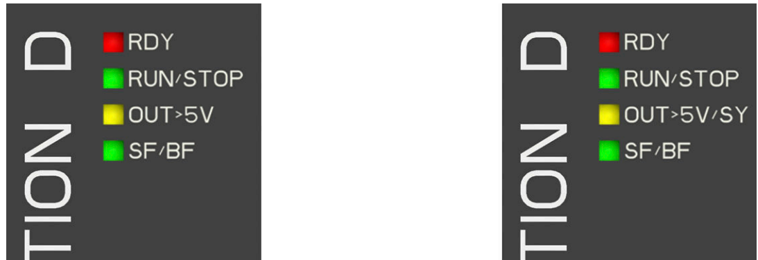
Figure 9-1 LED displays: D410-2 DP (pictured on the left), D410-2 DP/PN (pictured on the right)
