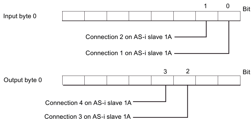
Figure 11-4 Assignment of the AS-i connections to the data bits of the input/output bytes
