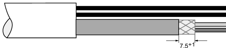
Figure 5-9 PROFIBUS Hybrid cable with heat-shrink tubing
