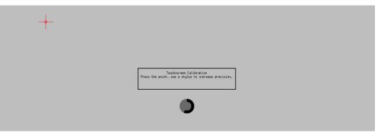
2. Briefly touch the center of the calibration crosshairs. A touch pen is recommended for calibration.
